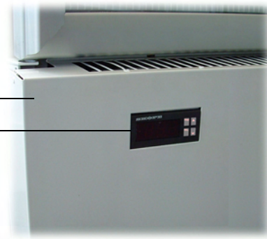
Figure 3: Electronic Controller Relocated
