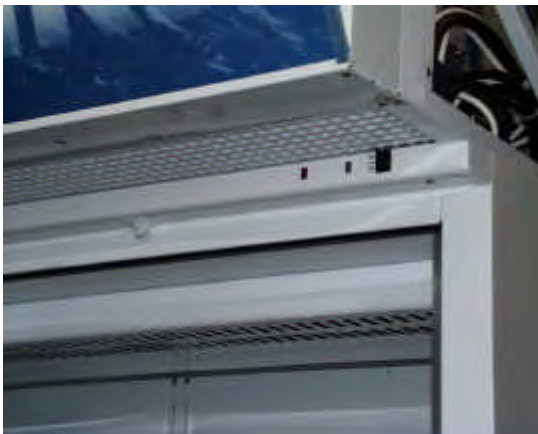
Figure 8: Door Activated Switch
