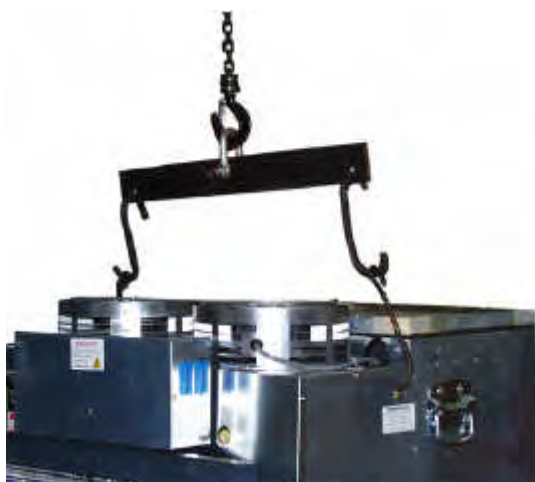
Figure 6: Mechanical Lifting of Unit
